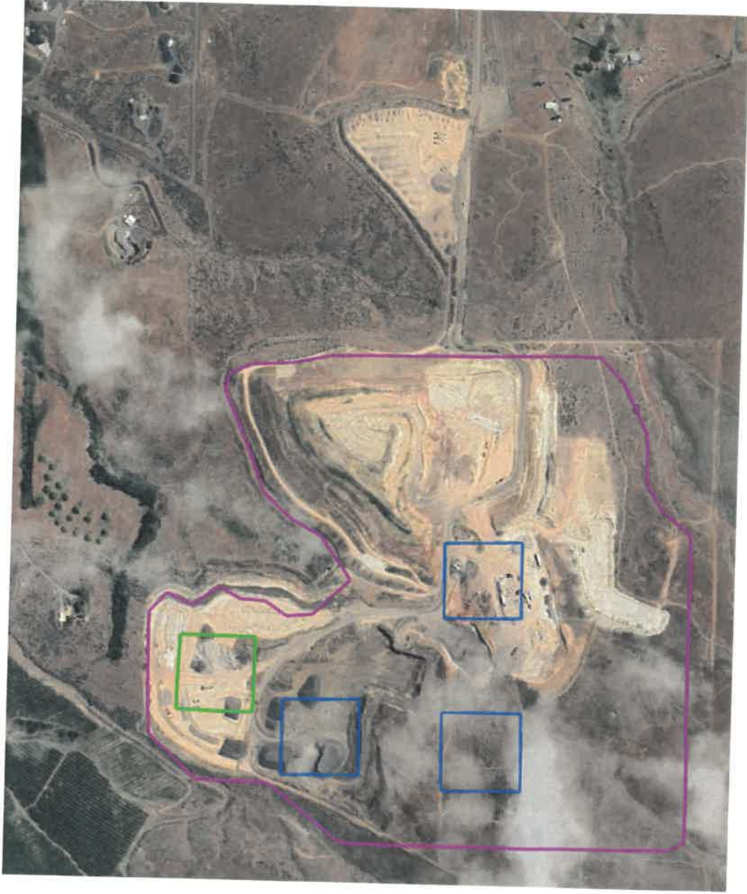
Figure 2: Permittee's proposed crusher location (outlined in green), and additional proposed modeled locations (outlined in blue), within the approved facility area (outlined in purple), where the crusher can be moved around without exceeding air emission thresholds.
