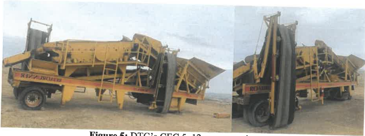
Figure 5: DTG's CEC 5x12 screen equipment.
